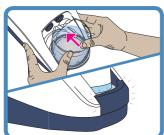
Fit the water chamber to the unit by pressing down the finger guard and sliding the chamber on, carefully aligning with the blue chamber port ends.
